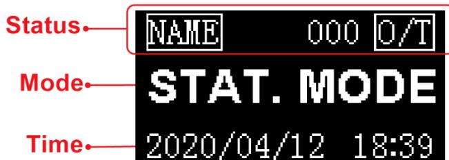
Here assumed that the operation mode is "Statistic", the printer with a lot of operation mode, different operation modes correspond to different uses and report styles, about the operation modes, please refer to the *Section 8*.
